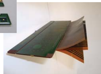
Photo 2: Two-layer flex-rigid wiring board (left); Flex-rigid multilayer (inner) wiring board
