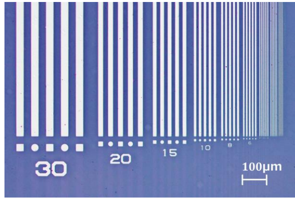
Wires ranging from 30 \mu\text{m} to 5 \mu\text{m} in width formed using the new technology
